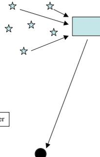
*Figure 5* illustrates one of the main differences between standard network RTK and PPP RT. In the case of PPP RTK the client user of the corrections can be at a great distance from the reference network.
