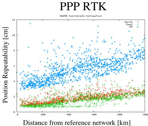
We investigated the quality of PPP RTK and standard PPP kinematic positioning as a function of the separation from a reference network. To do this we again estimated kinematic positions with a very loose 100 m /sec motion constraint every 30 seconds during 2 weeks for a large number of stations of Japan's GEONET.
