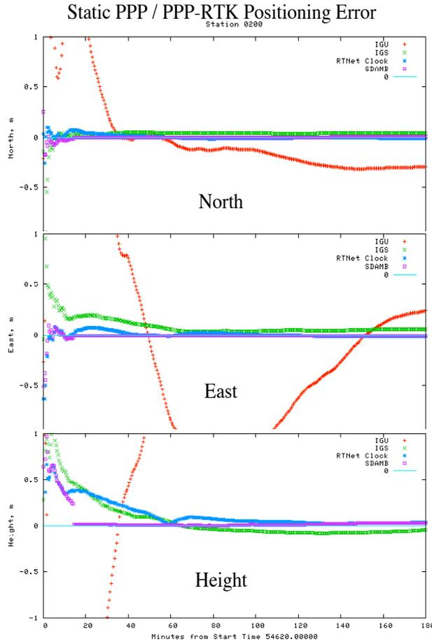
**Figure 2** This figure compares the initial 180 minutes of static positioning for GEONET station 0200. The solution modes that are compared are PPP with IGU predicted orbits and clocks (red), PPP with IGS final orbits and 30-sec clocks (green), PPP positioning with RTNet clocks (which are real-time improvements of the IGU clocks as described above) (blue) and PPP RTK solutions with RTNet determined MSCCs (purple).
