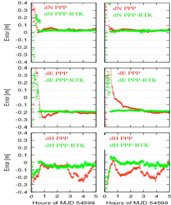
**Figure 3** compares PPP (red) and PPP RTK (green) positioning solutions for a fixed site that was estimated in kinematic mode. The first 5 hours of processing for two days (MJD 54598, 54599) are shown. The main points are the shorter convergence time and the more stable height component for the PPP RTK solution compared to the PPP solution.
