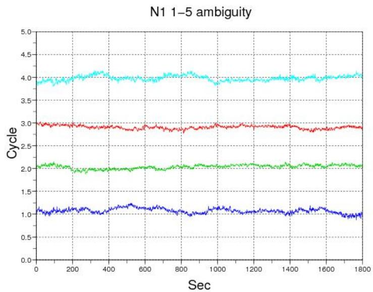
**Figure 7: ambiguity residuals for the N1 combination using fixed 1-5 widelane**
