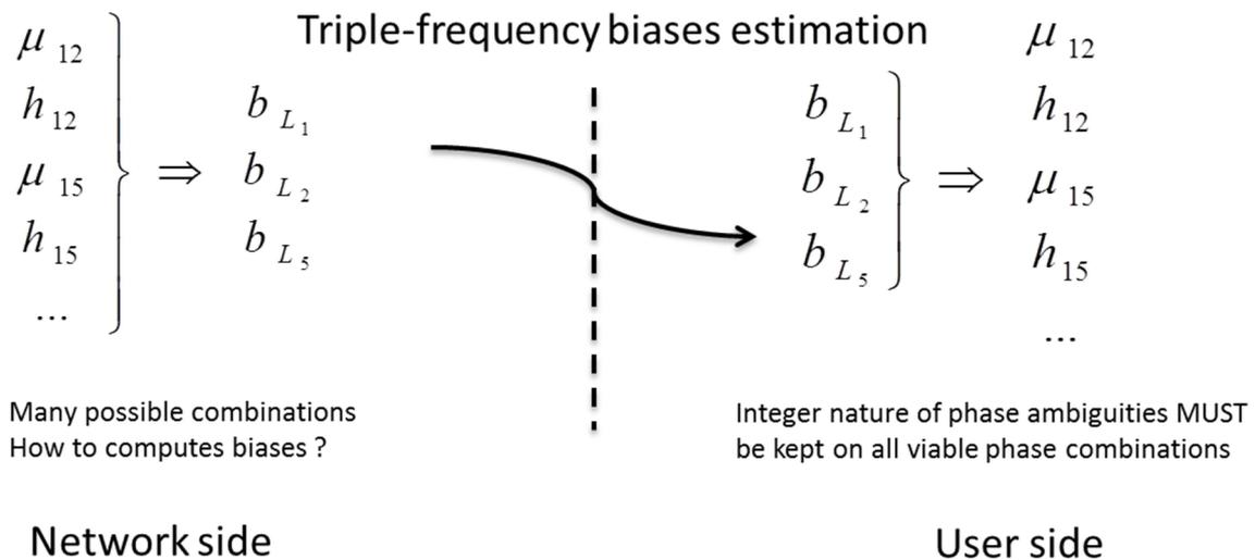
**Figure 2: phase biases estimation in the triple frequency case**
