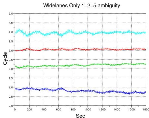
**Figure 5: ambiguity residuals for widelane-only ionosphere free combinations**
