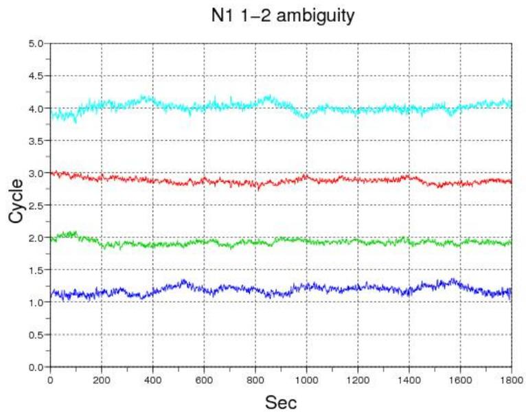
**Figure 6: ambiguity residuals for the N1 combination using fixed 1-2 widelane**
