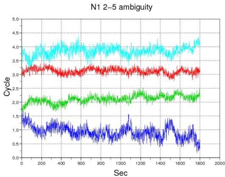
**Figure 8: ambiguity residuals for the N1 combination using fixed 2-5 widelane**
