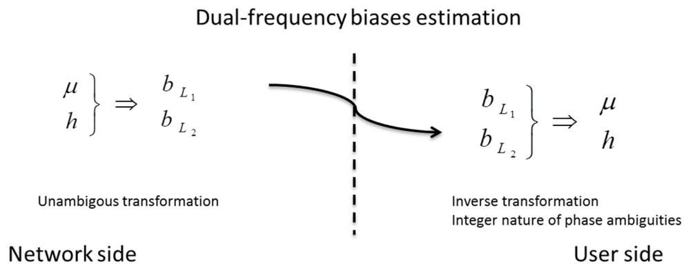
Figure 1: phase biases estimation in the dual frequency case
