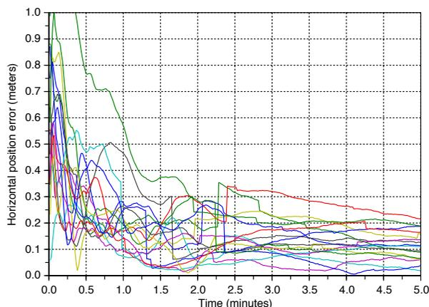
▲ FIGURE 10 Widelane-only triple-frequency PPP convergence (horizontal position error).
