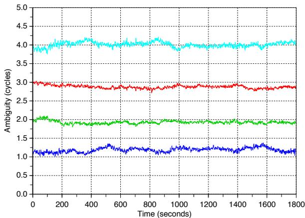
▲ FIGURE 6 Ambiguity residuals for the  $N_1$  combination using a fixed 1-2 widelane.
