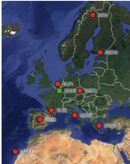
▲ FIGURE 9 Network used for the triple-frequency PPP study.
