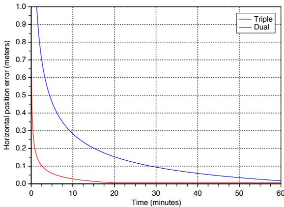
▲ **FIGURE 12** Realistic PPP convergence comparison between dual- and triple-frequency contexts (horizontal position error).
