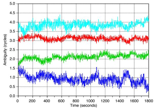
▲ FIGURE 8 Ambiguity residuals for the  $N_1$  combination using a fixed 2-5 widelane.
