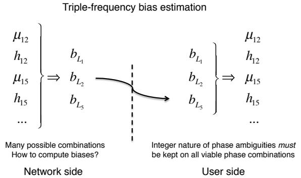
▲ FIGURE 2 Phase biases estimation in the triple-frequency case.
