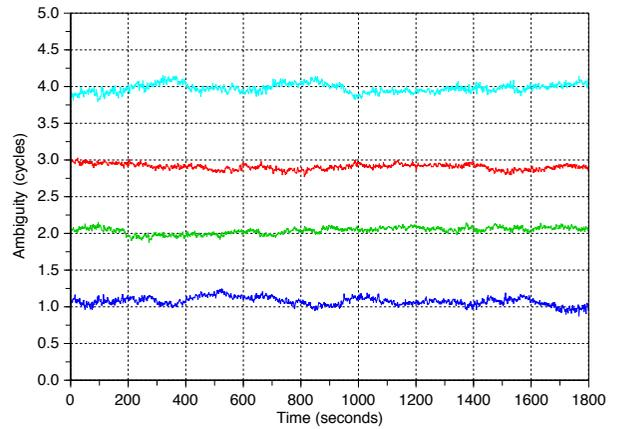
▲ FIGURE 7 Ambiguity residuals for the  $N_1$  combination using a fixed 1-5 widelane.
