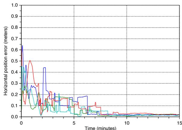
▲ FIGURE 11 All ambiguities triple-frequency PPP convergence (horizontal position error).
