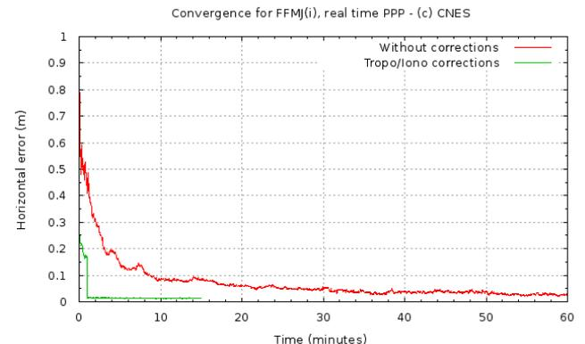
Figure 3: Typical dual-frequency PPP convergence
