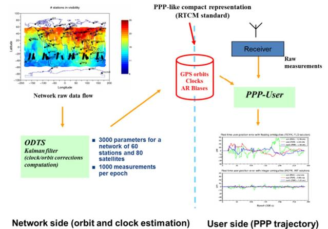
Figure 2: Typical PPP-AR architecture
