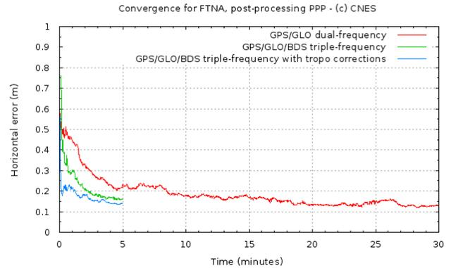
**Figure 13: Convergence figures in various configurations**
