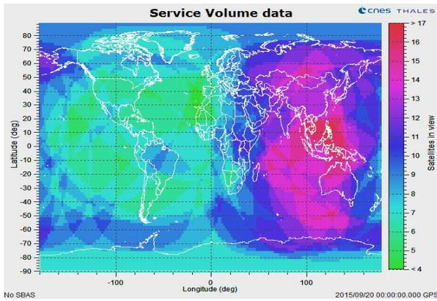
Figure 1: Number of triple frequency satellites in view
