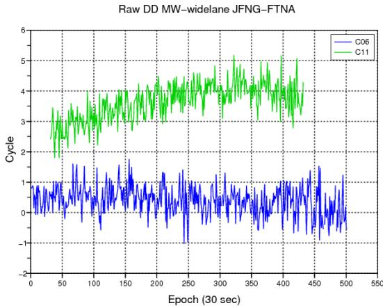
Figure 6: Raw Beidou MW-DD
