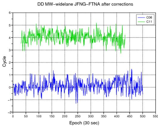
Figure 7: Bias-corrected Beidou MW-DD
